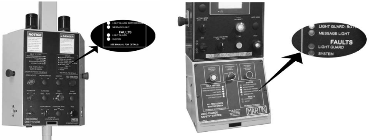
Figure 2 – Retrofit & “Boom Buddy” Fault & Message Lights (023375/6.jpg)
