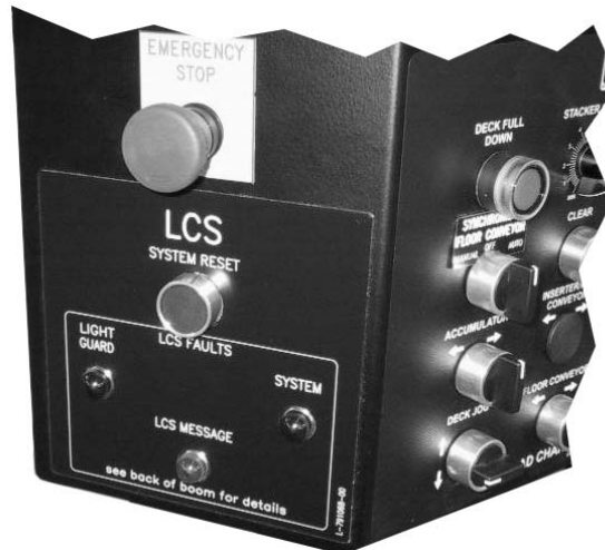
Figure 3 – New LCS-Series Stacker Fault & Message Lights (023379.jpg)
